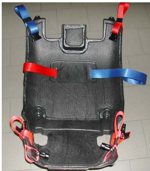
Figure 3. Disposition of strap receptacles
