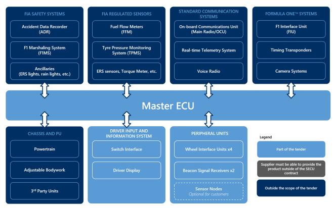
Together, the on-car SECU hardware and software must be able to support all electro-mechanical systems running on a car designed according to the Formula One regulations. In 2020, these include the hybrid Power Unit, Gearbox, Clutch and Differential that constitute current F1 powertrains as well as the Adjustable Bodywork, Brake System and Tyre Monitoring System of the car.
