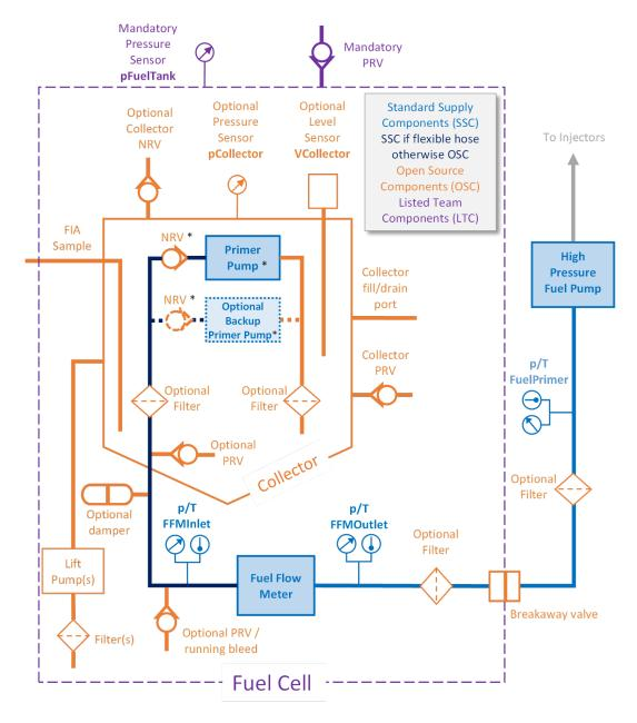
**6.6.5** If a fuel pressure damper is fitted it must be fitted upstream of the Fuel Flow Meter described in article 5.11.3.
