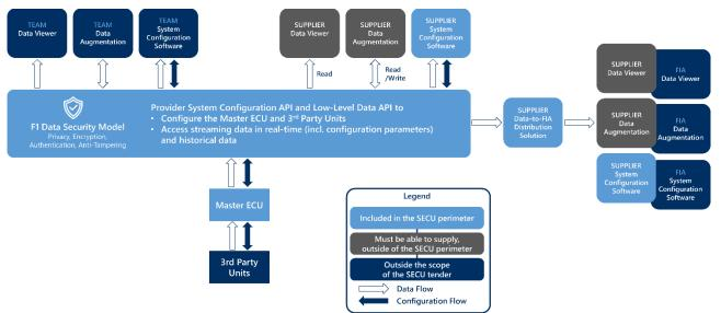
Streamlining the access to data should be achieved by providing a set of Applications Programming Interfaces (APIs). The above diagram shows how these APIs may be integrated within a typical trackside Formula 1 data platform. Note that the various software applications and tools interfacing with the Master ECU through this set of APIs are expected to be either supplied by the provider, developed in-house by the various stakeholders or subcontracted to third-parties.
