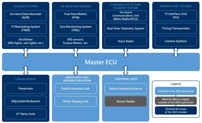
Together, the on-car SECU hardware and software must be able to support all electro-mechanical systems running on a car designed according to the Formula One regulations. These include the hybrid Power Unit, Gearbox, Clutch and Differential that constitute current Formula One powertrains as well as the Adjustable Bodywork, Brake System and Tyre Monitoring System (TMS) of the car.
