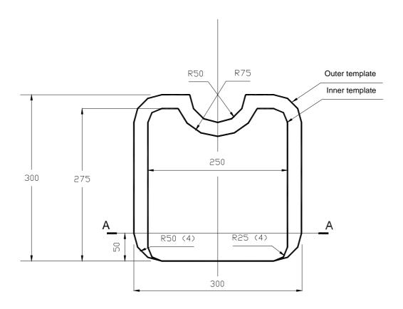
Drawing 3: Cockpit cross section template
