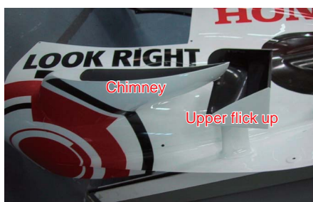
Fig. 28 Chimney and upper flick-up
