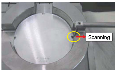
Fig. 11 Expanded ring taper angle measurement jig
