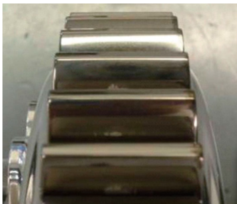
Fig. 13 Final gear condition after 4 races
