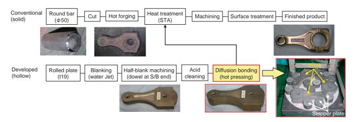
Fig. 3 Developed process of manufacture of hollow connecting rod
