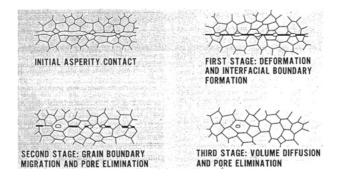
Fig. 1 Model of diffusion bonding process
