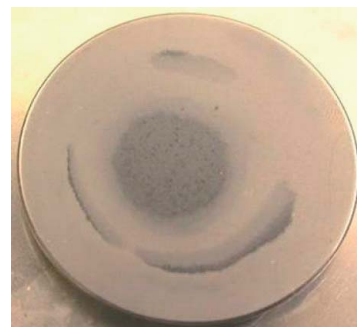
Fig. 2 Segregation structure of valve
