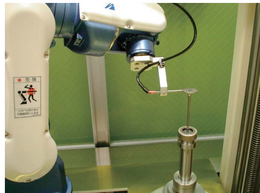
Fig. 4 Method of eddy current inspection
