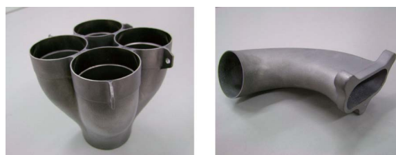
Fig. 7 Casting collector and primary transitional pipe
