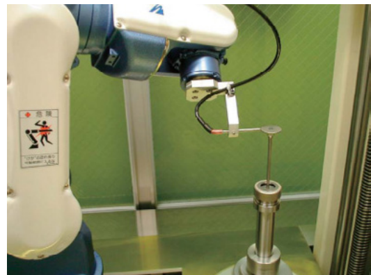
Fig. 4 Method of eddy current inspection
