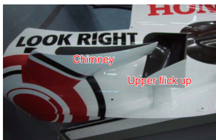
Fig. 28 Chimney and upper flick-up
