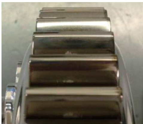
Fig. 13 Final gear condition after 4 races
