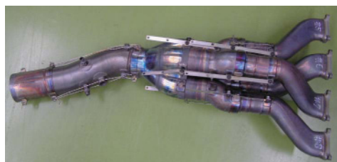
Fig. 24 Test exhaust system
