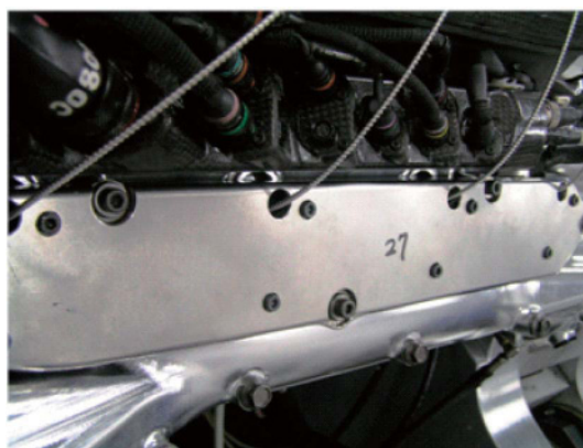
Fig. 4 Photograph of overview of cylinders to which micro-Cassegrain sensors were attached
