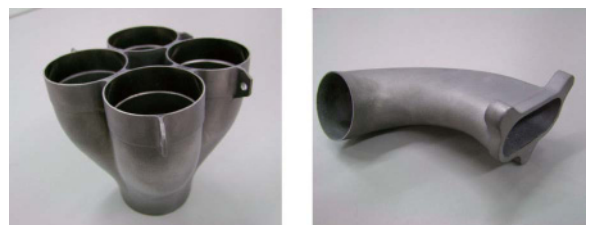
Fig. 7 Casting collector and primary transitional pipe
