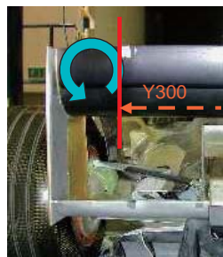
Fig. 39 Secondary vortex due to RW load distribution
