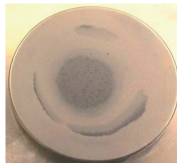
Fig. 2 Segregation structure of valve
