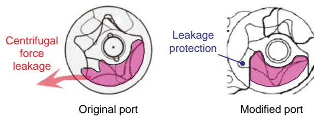
Fig. 16 Comparison of suction port shape (shown as pink area)
